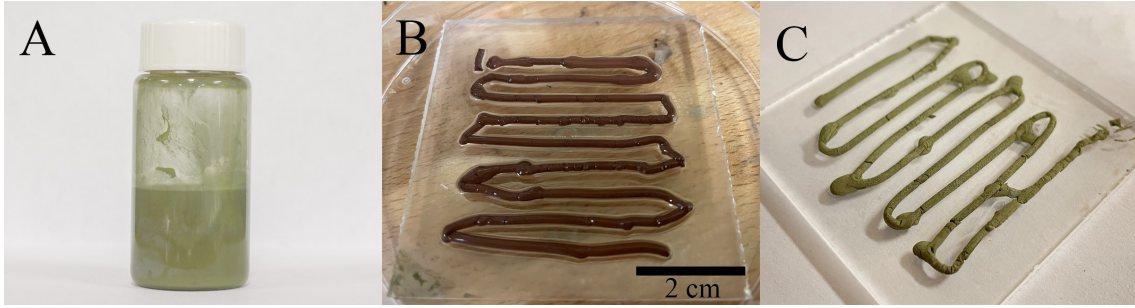
Figure 3.1: Stages of the printing process: Energetic \text{GO}(20\%)/\text{Al}/\text{Bi}_2\text{O}_3 nanothermite ink (A) as printed \text{rGO}(20\%)/\text{Al}/\text{Fe}_2\text{O}_3 organogel (B) and post-freeze dried \text{rGO}(20\%)/\text{Al}/\text{Bi}_2\text{O}_3 aerogel (C).
