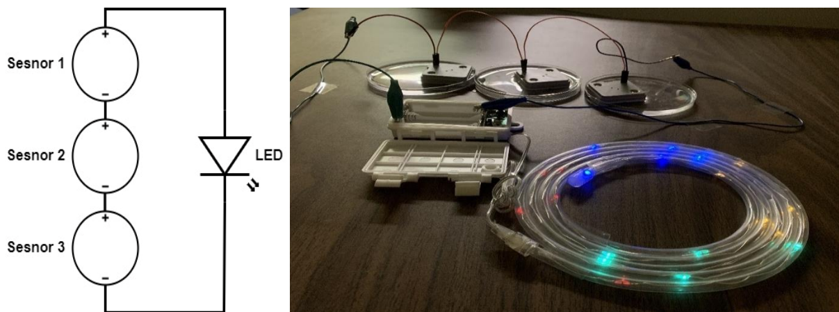
Figure 22: Three Sensors connected in series with LED.
