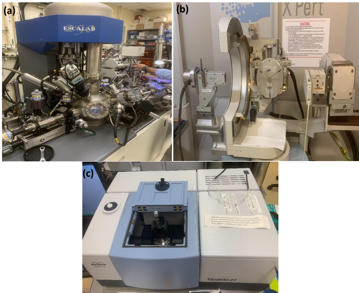
Figure 12: (a) XPS Instrument; (b) XRD Machine; (c) ATR-FTIR Spectroscopy (pictures taken while doing the measurement).
