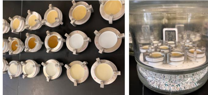
Figure 3.7 The condition of WVP test.
