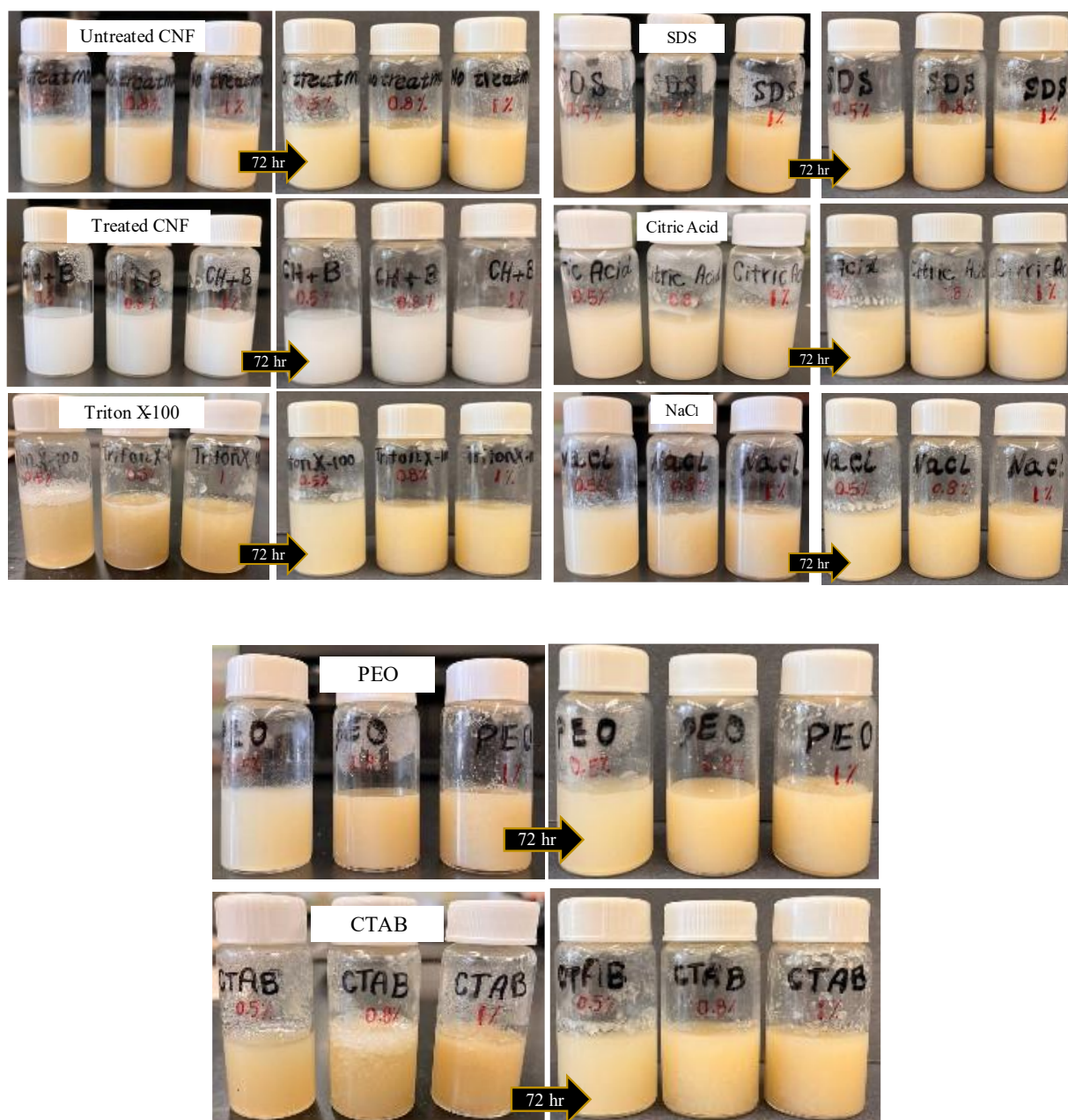
Figure 6.5 Visual dispersibility after sonication as a function of concentration of CNF.
