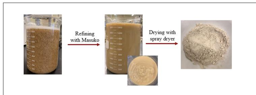
Figure 3.3 Making CNF without chemical treatment.
