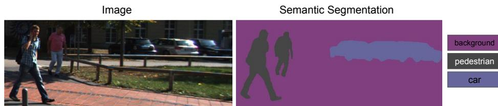
Figure 3.1: An example of semantic segmentation for an input image. Each pixel is assigned a class label from the ‘background’, ‘car’, and ‘pedestrian’ classes.
