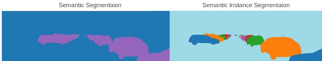
Figure 1.1: Comparison of semantic segmentation and semantic instance segmentation. On left, dark blue shows ‘background’ class, purple shows ‘car’ class and light blue shows ‘bicycle’ class. On right, light blue shows the background. Other colors are random for distinguishing different object instances. Note that in instance segmentation there is an object class predicted for each mask as well, such as ‘car’, ‘pedestrian’, or ‘bicycle’, which is not shown in the figure for simplicity.
