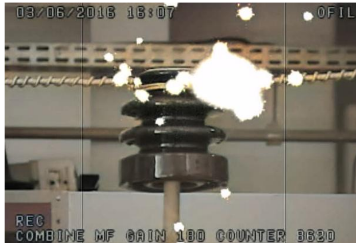
Figure 1.8 UV camera measurement of a drilled contaminated insulator sample [21]
