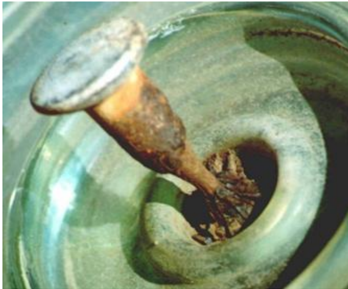
Figure 1.4 Pin corrosion due to improper stress grading and high contamination [11]
