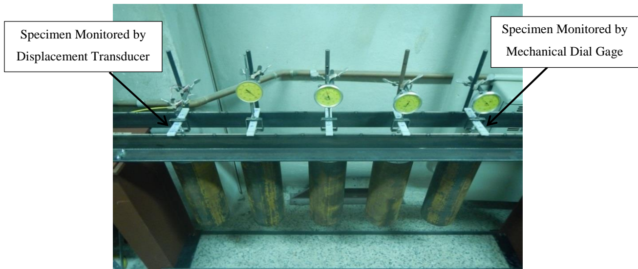
Figure 6.5 - Typical flexural creep test setup
