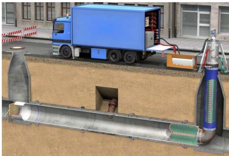
Figure 2.5 - CIPP installation process ( Unitracc , 2013)
