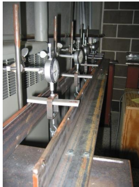
Figure 2.10 - End view of specimens under creep load (Adapted from CATT Report , 2005)
