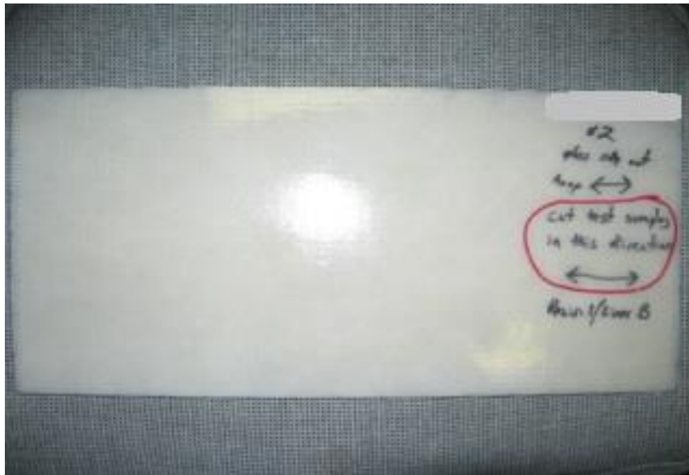
Figure 3.1 - Front view of a typical CIPP plate ("as received condition")
