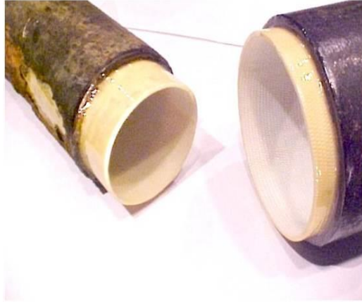
Figure 2.6 - CIPP liner cured inside a deteriorated pipe (Adapted from Knight , 2013)
