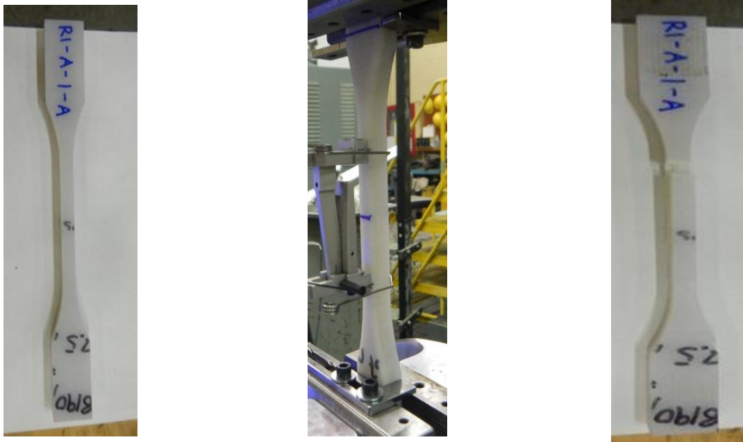
Figure 4.2 - Liner "A" specimen, before, during, and after the tensile test
