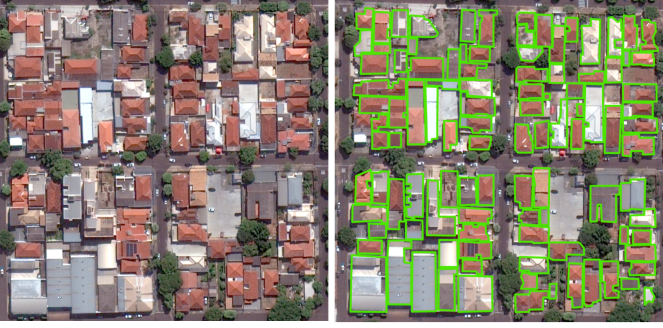
Fig. 2. Sample of the roof areas considered in the case study, determined using GIS tools.
