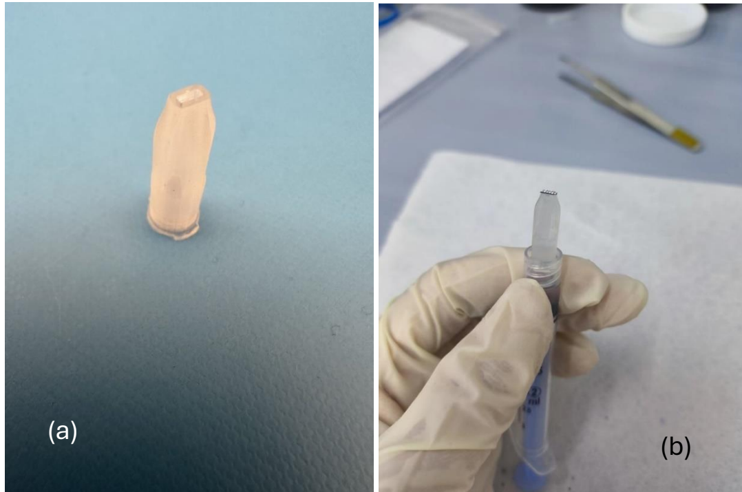
Figure 4.28 Microneedle test device manufacturing. (a) Polymer applicator fabricated by 3D printing; (b) Microneedle chip connecting syringe with applicator.
