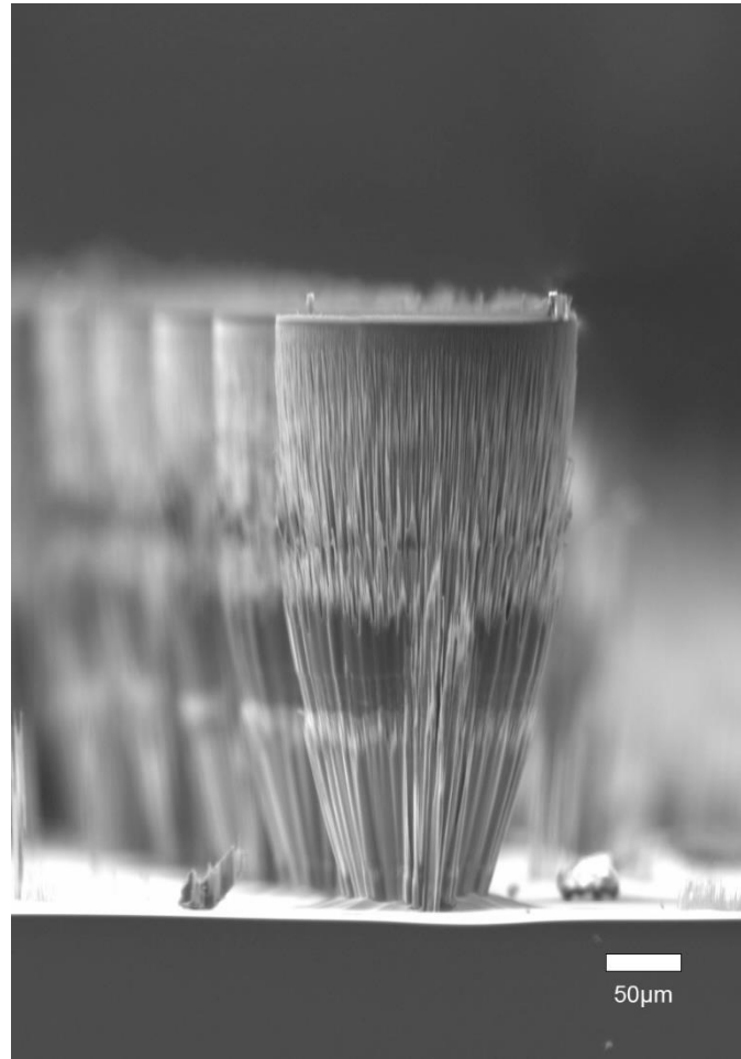
Figure 4.22 Pillar structures etched without sacrificial structures.
