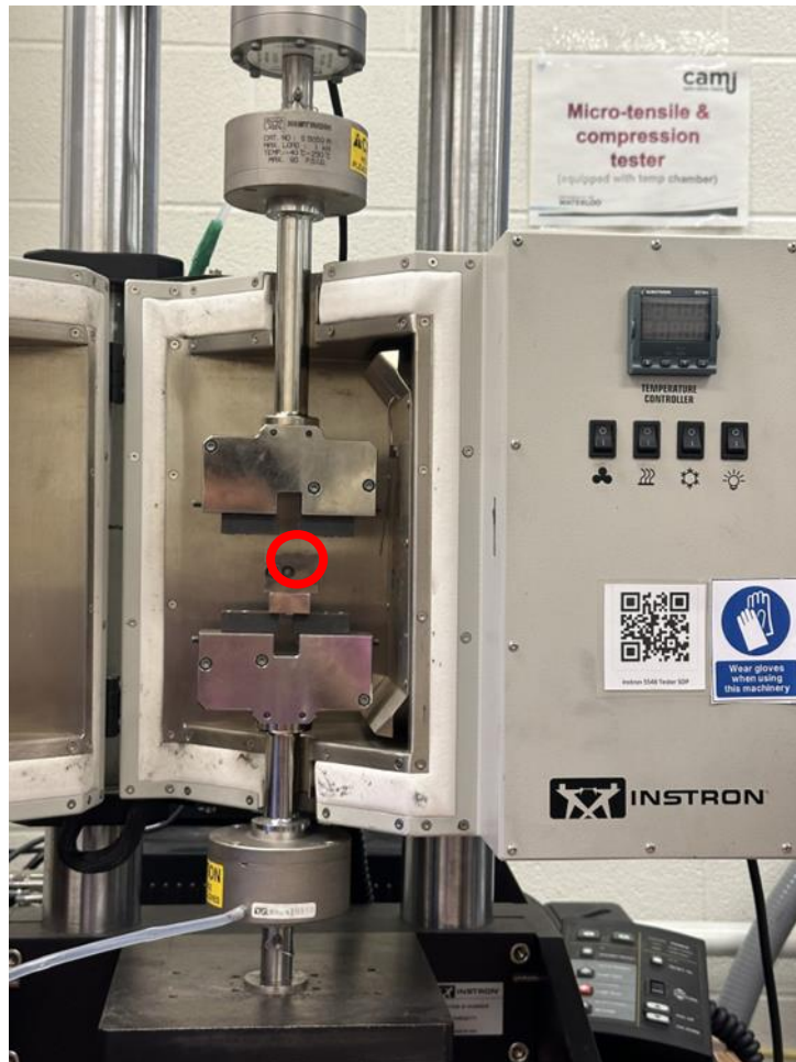
Figure 4.33 Instron 5548 micro tester. The microneedle chip is placed on the platform (circled area).
