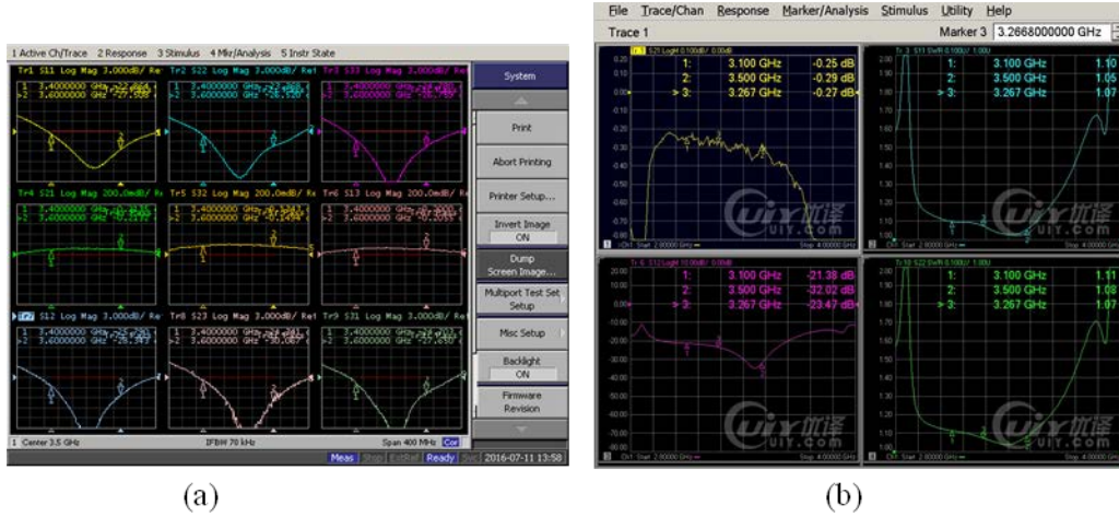
Figure 3-2 Two examples of performance characterization for commercial Sub-6 GHz circulators obtained directly from the manufacturers, (a) JQL Circulators ( www.jqlelectronics.com ) and (b) UIY Circulators ( www.uiy.com ).
