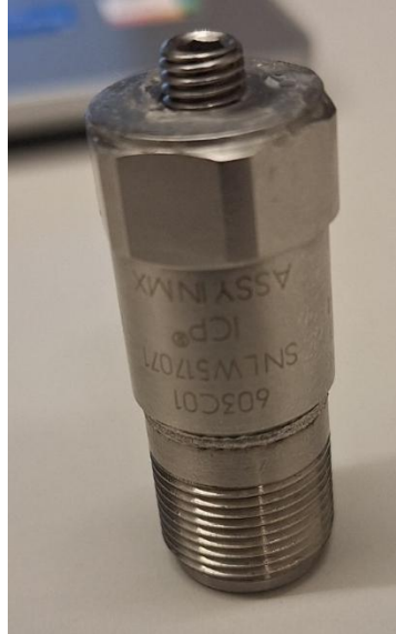
Appendix A 1 Uniaxial ICP® accelerometer (model 603C01) used for vibration data collection on the jackleg drill.
