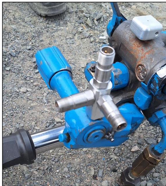
Figure 5.5-1 Mounted accelerometers on the Handle of the drill, showing orientation relative to the structural axis.
