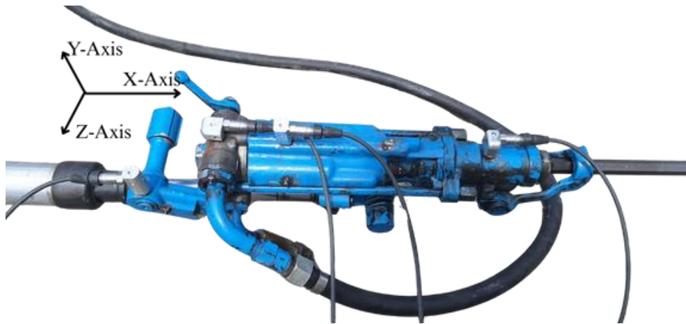
Figure 4.4-1 top view of the jackleg drill instrumented with accelerometers at multiple locations, and X, Y & Z axes defined.
