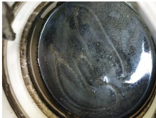
Figure 14. A DI water and powder mixture of a 4%wt activated carbon batch
