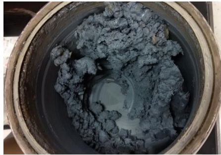
Figure 16. Finished paste with PTFE emulsion addition in a mixing bowl
