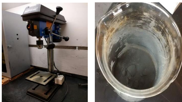
Figure 12. Drill press mixing machine and mixed dry powder
