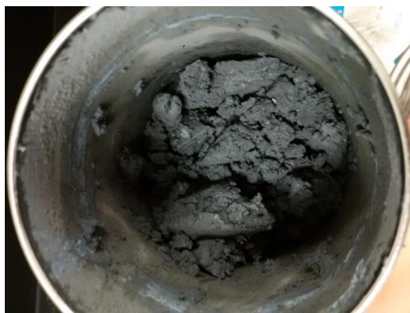
Figure 15. The paste in the mixing bowl after the sulfuric acid addition
