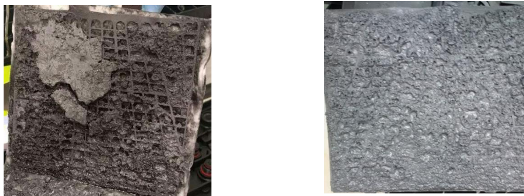
Figure 35. Negative electrode without binder (right) after 20 cycles and with PTFE as binder (left) after
