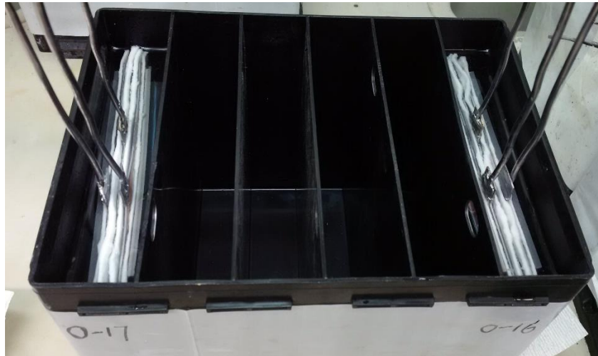
Figure 23. Soaking assembled cells in the battery box
