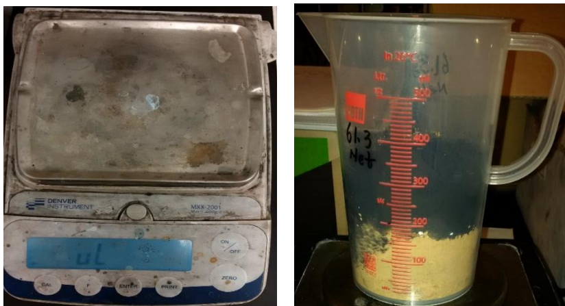
Figure 11. Balance for weighting solids and solids Measuring in a cup
