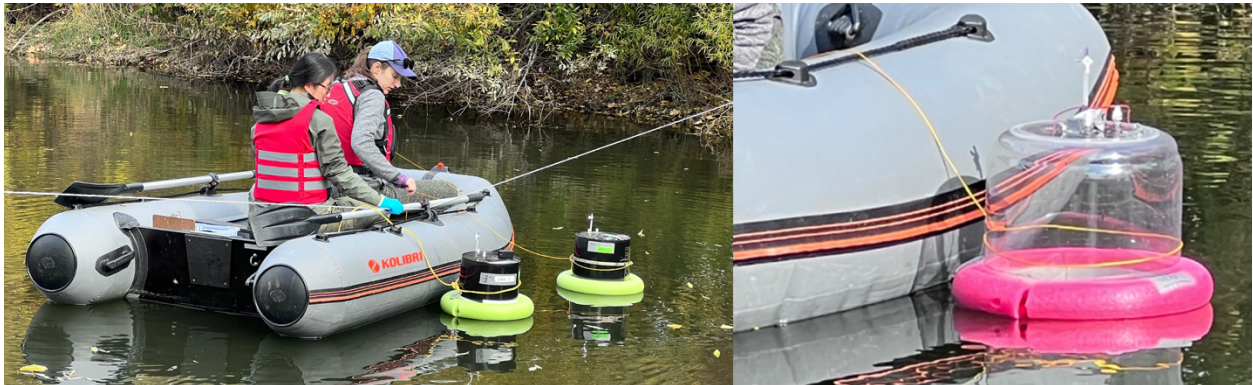
Figure AI-2: Clear and dark floating chamber setup for open water flux measurements. Chambers were deployed from an inflatable boat and anchored during each measurement.
