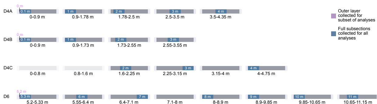
Figure 5.2 Schematic of the ~1 m core segments retrieved and the subsamples that were collected for analysis (purple and blue). Light grey cores represent depths that were not analyzed for microbiology.
