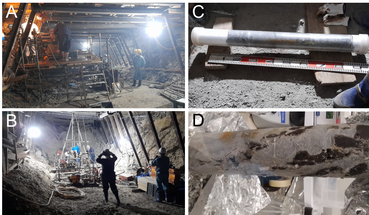
Figure 5.1 Photo of the drilling setup at the site where the D4 (A) and D6 (B) cores were retrieved, an example of a core in its acrylic casing (C) and once removed from the acrylic casing (D).
