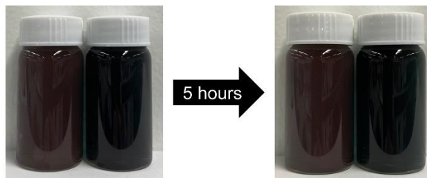
Figure 5.6 Aqueous suspension stability of (left) CNC/PEI/Cu and (right) CNC/PEI/ \text{Cu}_2\text{O} over 5 h.
