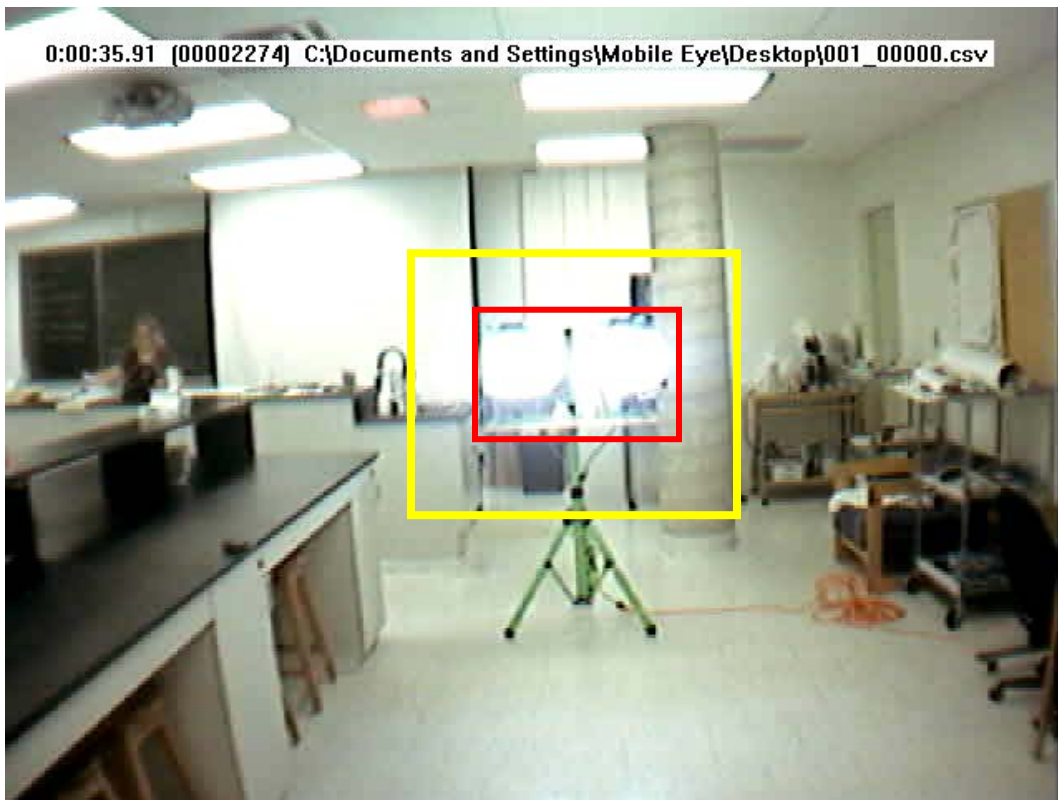
Figure 7. The three zones of distinction for determining if a participant was looking into, slightly away or away from the glare source.
