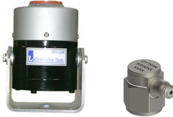
Figure 2.3: electrodynamic shaker (Labwork Inc. ET-126B-1) and Accelerometer (Dytran 3055B3)
