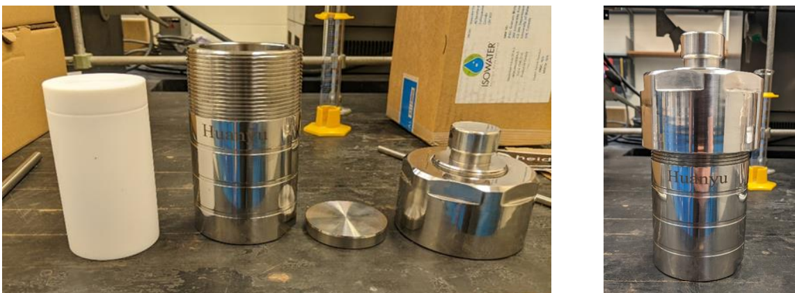
Figure 2-20: Teflon cup insert and disassembled stainless steel jacket of hydrothermal autoclave reactor (left) and sealed reactor (right).
