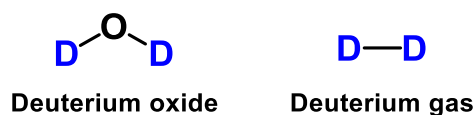
Figure 1-2: Deuterated forms of water and hydrogen gas, common industrial sources of deuterium.
