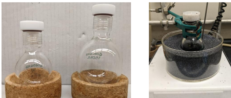
Figure 2-17: Glass pressure vessels (left) used for preliminary reactions with heterogeneous catalyst stirred as a slurry at high temperature (right).
