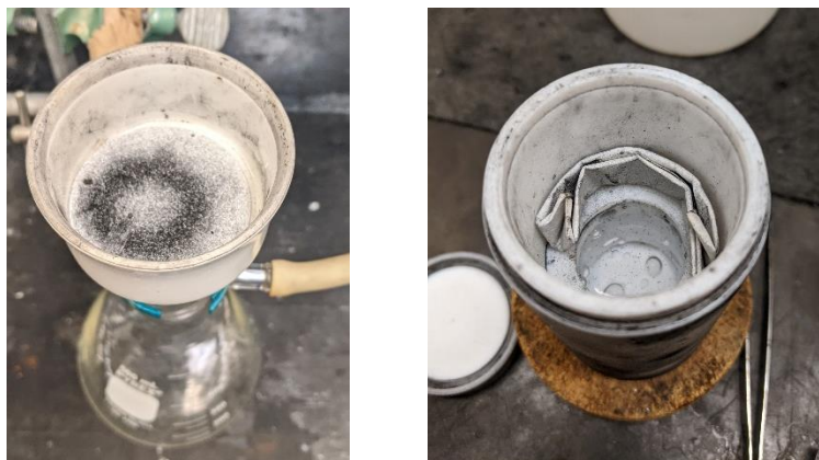
Figure 2-19: The catalyst medium is prepared by dispensing Pt/C as a slurry on filter paper under vacuum suction and dried before using (left). The filter paper is placed inside the Teflon liner on a stand to keep it above the liquid surface (right), folding the filter paper allows for larger filter papers to fit inside and does not impact reactivity.
