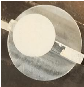
Figure 4-5. Manually blade coated bi-layer membrane (NiO-BZCY172-starch|BZCY172) stick on stainless stub, the white paste is coated on pre-sintered substrate
