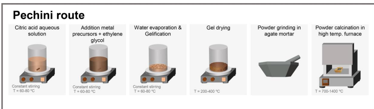
Figure 1-7. Illustration of the steps involved in the Pechini route (Reprinted from [30] with permission from Springer Nature)
