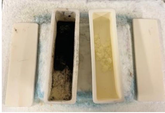
Figure 3-1. the white solid material before combustion in the alumina crucible (right), and after combustion at 200°C for 3 hours (left)
