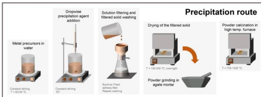
Figure 1-9. Illustration of the steps involved in the precipitation route (Reprinted from [30] with permission from Springer Nature)
