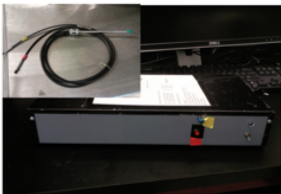
(a) Optical probe with fluorometer setup.
