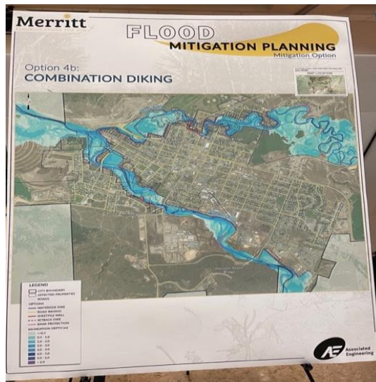
Figure 2: Flood mitigation plans developed by Associated Engineering for Merritt. a A flood mitigation plan depicts 4 comprehensive options that is showcased to the public at a flood recovery open house in June 2022. b Option 2 categorized as a full floodplain retreat is graphically represented on a flood map. c Option 3 represented as waterside diking is shown on a flood map. d Option 4a categorized as combination diking includes the raising of roads and setback dikes. e Option 4b includes setback dikes behind the mobile home park. f Option 4c includes waterside diking upstream of the Houston Street Bridge (Cottar, 2022).
