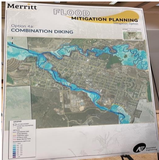
Figure 2: Flood mitigation plans developed by Associated Engineering for Merritt. a A flood mitigation plan depicts 4 comprehensive options that is showcased to the public at a flood recovery open house in June 2022. b Option 2 categorized as a full floodplain retreat is graphically represented on a flood map. c Option 3 represented as waterside diking is shown on a flood map. d Option 4a categorized as combination diking includes the raising of roads and setback dikes. e Option 4b includes setback dikes behind the mobile home park. f Option 4c includes waterside diking upstream of the Houston Street Bridge (Cottar, 2022).
