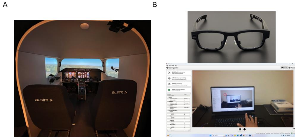
Figure 6.1. Illustration of the simulator and eye tracking equipment set-up. The ALSIM simulator was set up as a single-engine aircraft, controlled with the yolk, throttle lever, and rudders pedals (A). Participants also used a headset (hanging on the left window) to make ATC calls (A). The AdHawk glasses (B) were worn by participants throughout the experimental session and were connected to the collection laptop (B) via a USB-C cord. The collection laptop used AdHawk software to calibrate the eye tracker and start and stop eye tracking data collection.
