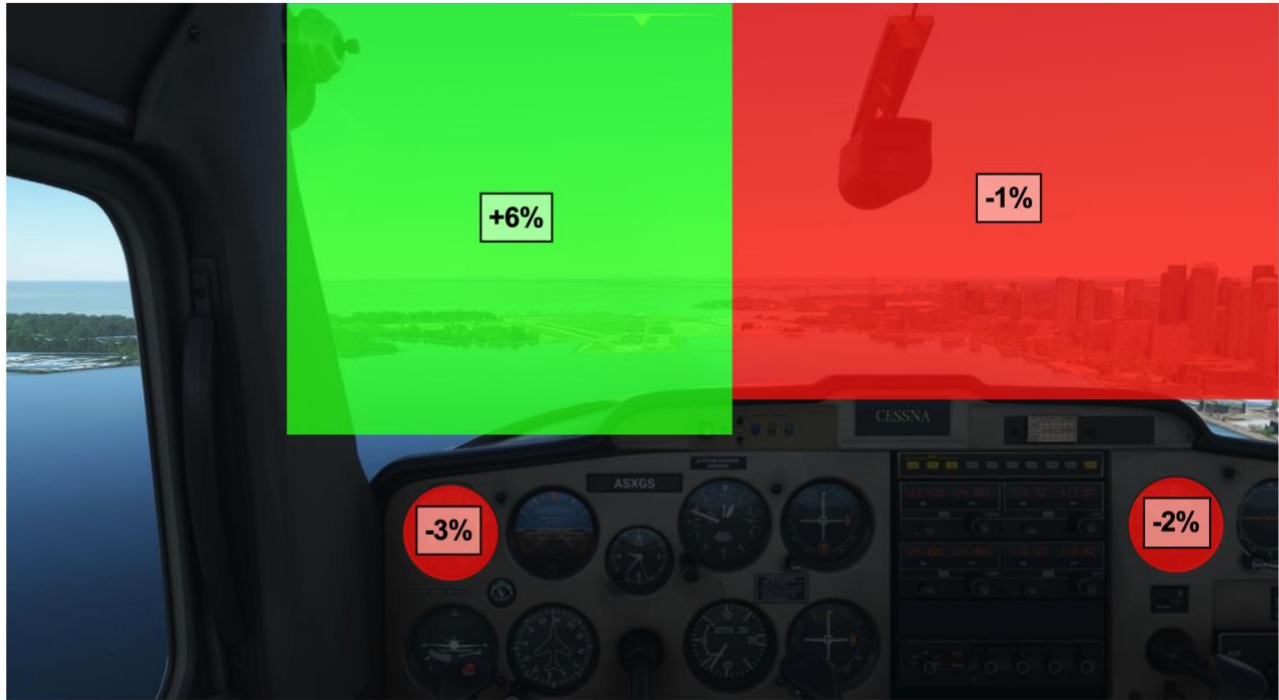
Figure 5.4. Illustration of the visual stimuli employed during landing and the corresponding change in dwell time (%) between easy and difficult conditions. Only significant changes in dwell time are displayed over their corresponding area of interest (AOI) (i.e., airspeed, power, runway, and horizon AOIs). Group mean differences (difficult-easy) are illustrated in red to indicate a decrease in AOI dwell time and green to indicate an increase in AOI dwell time.
