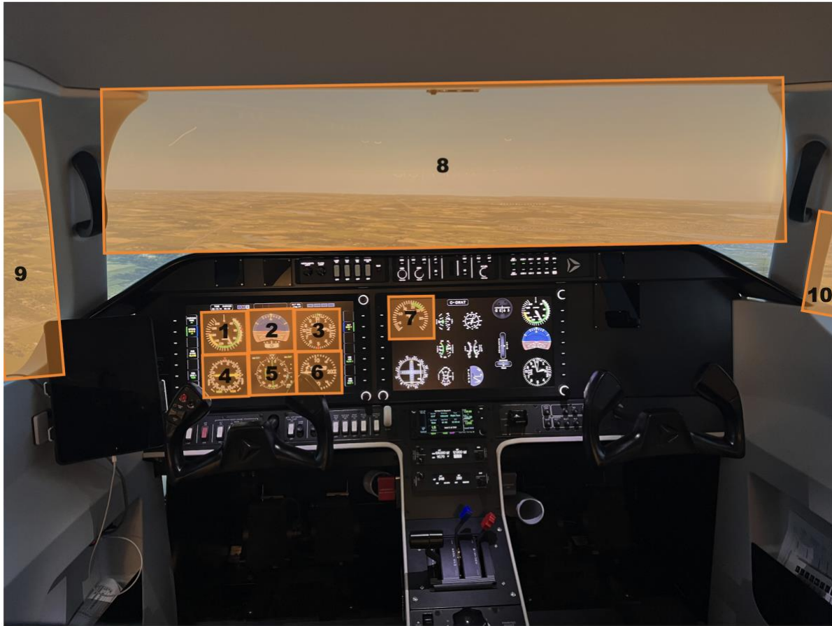
Figure 8.1. Illustration of the visual stimuli employed in the AL250 flight simulator environment. The participants point of view of the cockpit replicated that of a pilot flying a Cessna 172, pre-set for a cruise and landing approach to Waterloo International Airport, Breslau, Ontario, CA. The orange boxes represent the ten main areas of interest used in the gaze analyses. These include the airspeed (1), attitude (2), altimeter (3), turn coordinator (4), heading (5), vertical speed (6) and power (7) indicators, as well as the front (8), left (9), and right windows (10).
