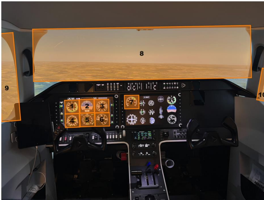
Figure 6.3. Illustration of the visual stimuli employed in the AL250 flight simulator environment. The participants point of view of the cockpit replicated that of a pilot flying a Cessna 172, pre-set for a downwind-to-base-to-final approach to Waterloo International Airport, Breslau, Ontario, CA. The orange boxes represent the ten main areas of interest used in the gaze analyses. These include the airspeed (1), attitude (2), altimeter (3), VOR (4), heading (5), vertical speed (6) and power (7) indicators, as well as the front (8), left (9), and right windows (10).
