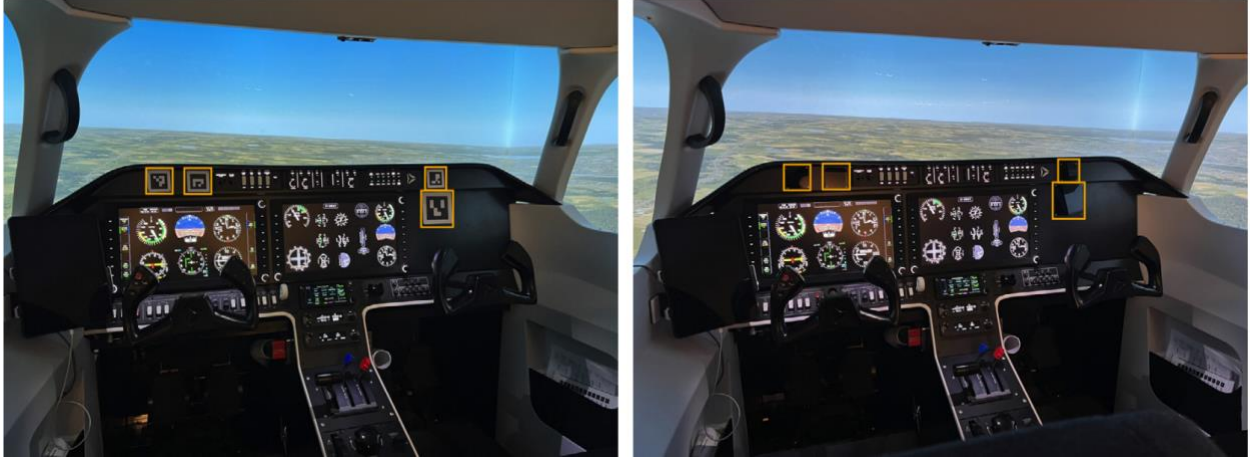
Figure 7.1. Illustration of the ArUco marker placement within the flight simulator for both visible (left) and invisible (right) marker types.
