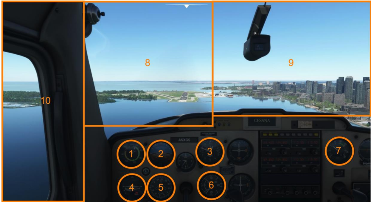
Figure 5.1. Illustration of the visual stimuli employed in the Microsoft Flight Simulator landing challenge environment. The participants point of view of the cockpit replicated that of a pilot flying a Cessna 152, pre-set for a straight-on approach to Billy Bishop airport, Toronto, Canada. The orange boxes represent the ten main areas of interest used in the gaze analyses. These include the airspeed (1), attitude (2), altimeter (3), turn coordinator (4), heading (5), vertical speed (6) and power (7) indicators, as well as the runway (8), horizon (9), and side window (10).
