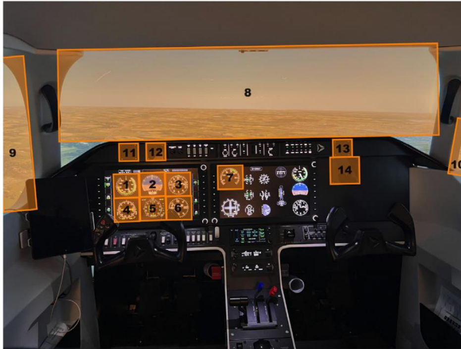
Figure 7.4. Illustration of the visual stimuli employed in the simulator environment. The participant's point of view in the cockpit was pre-set for a downwind-to-base-to-final approach to Waterloo International airport, Breslau, ON, Canada. The orange boxes represent the fourteen Areas Of Interest used in the gaze analyses. These include the (1) airspeed, (2) attitude, (3) altitude, (4) VHF Omni Range (VOR), (5) heading, (6) vertical speed, (7) power, as well as (8) the front window, (9) left window, (10) right window. The additional 4 Areas of Interest (11-14) represent the four markers that were placed in the cockpit around the instrument panel for optimal camera detection.
