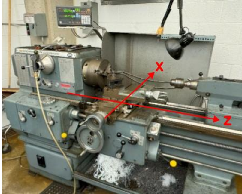
Figure 4.5: Manual lathe used for the orthogonal analogy wear tests.
