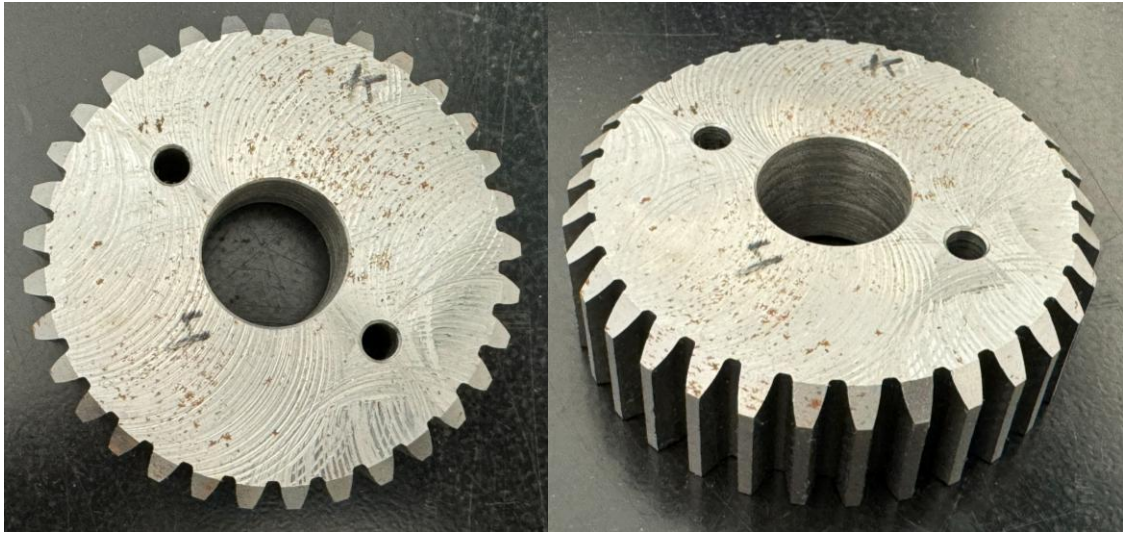
Figure 3.18: Sample gear produced using the five-axis milling machine.
