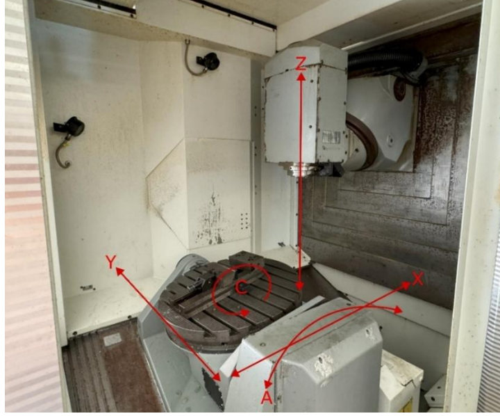
Figure 3.2: Motion axes of the five-axis CNC milling machine.
