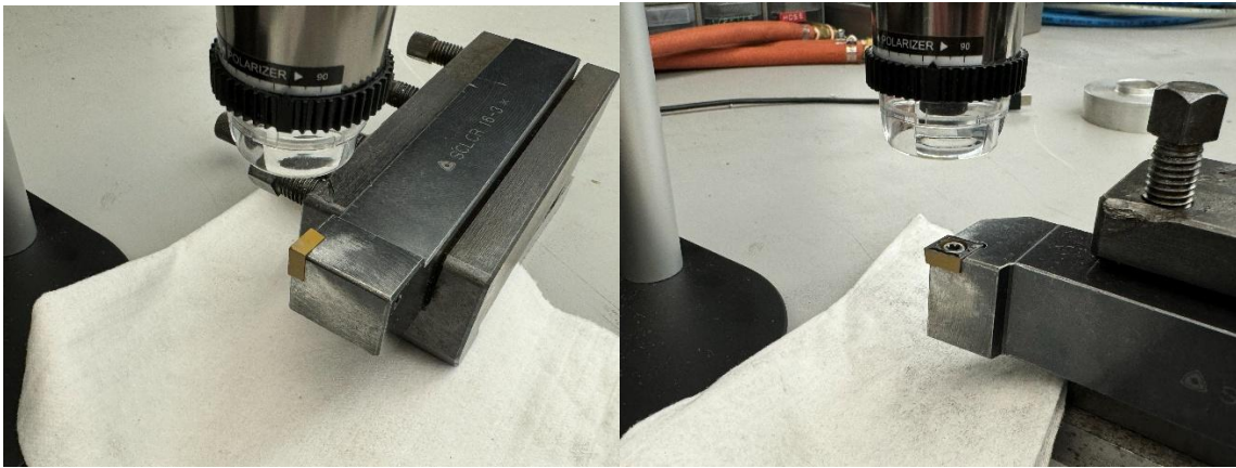
Figure 4.6 : Measurement setup for flank wear on the flank face of the cutting insert.
