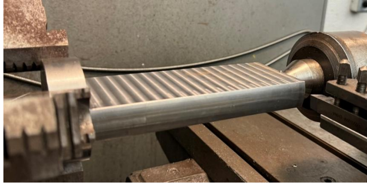
Figure 4.2: Initial design of the workpieces used for the orthogonal cutting analogy test.
