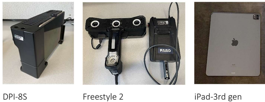
Figure 3-6: 3D scanning systems used at the RCM stores to scan components.
