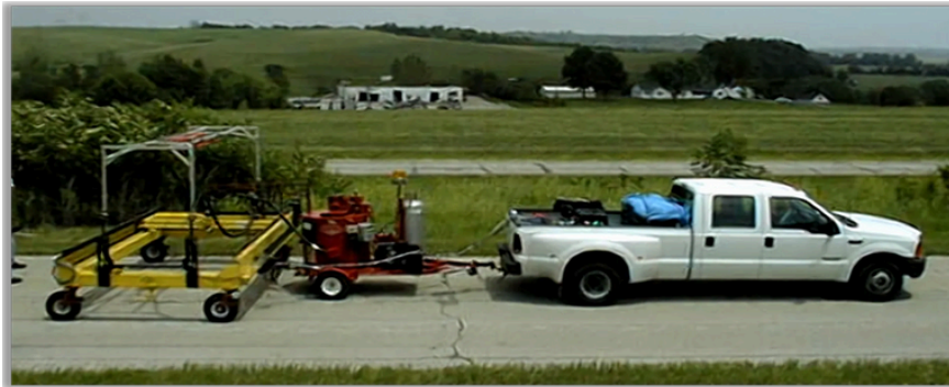
Figure 11 - Final version in the series of the CMU-UT automated crack sealing systems, demonstrated in ten states in 1999
