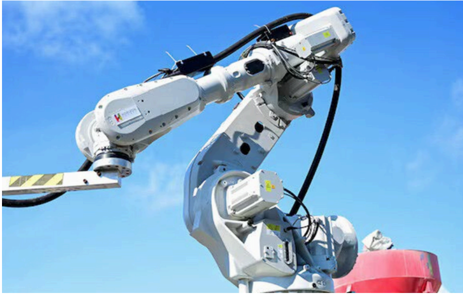
Figure 15 - 3D concrete printing. Used with permission. (Horizon Legacy. 2025).
