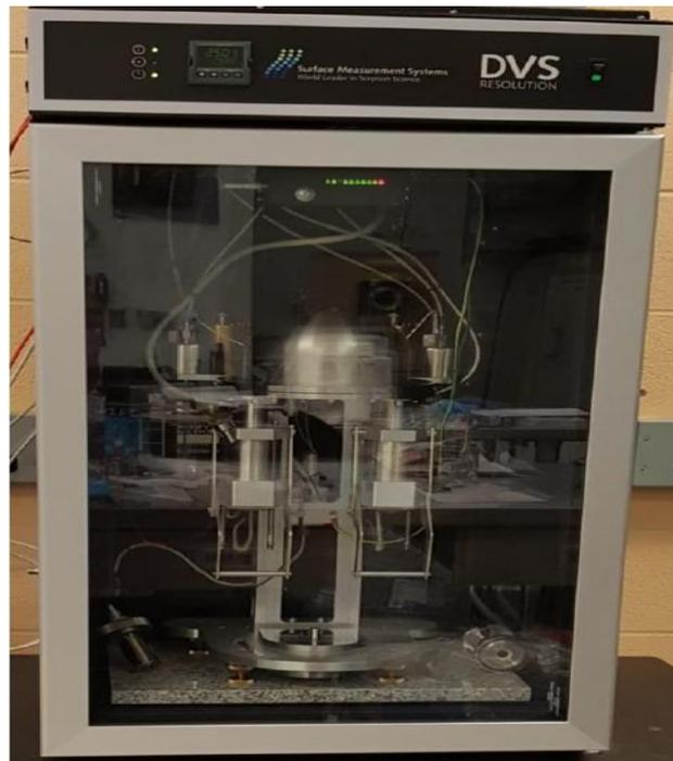
*Figure 2-11 – Dynamic vapor sorption (DVS) resolution device*
