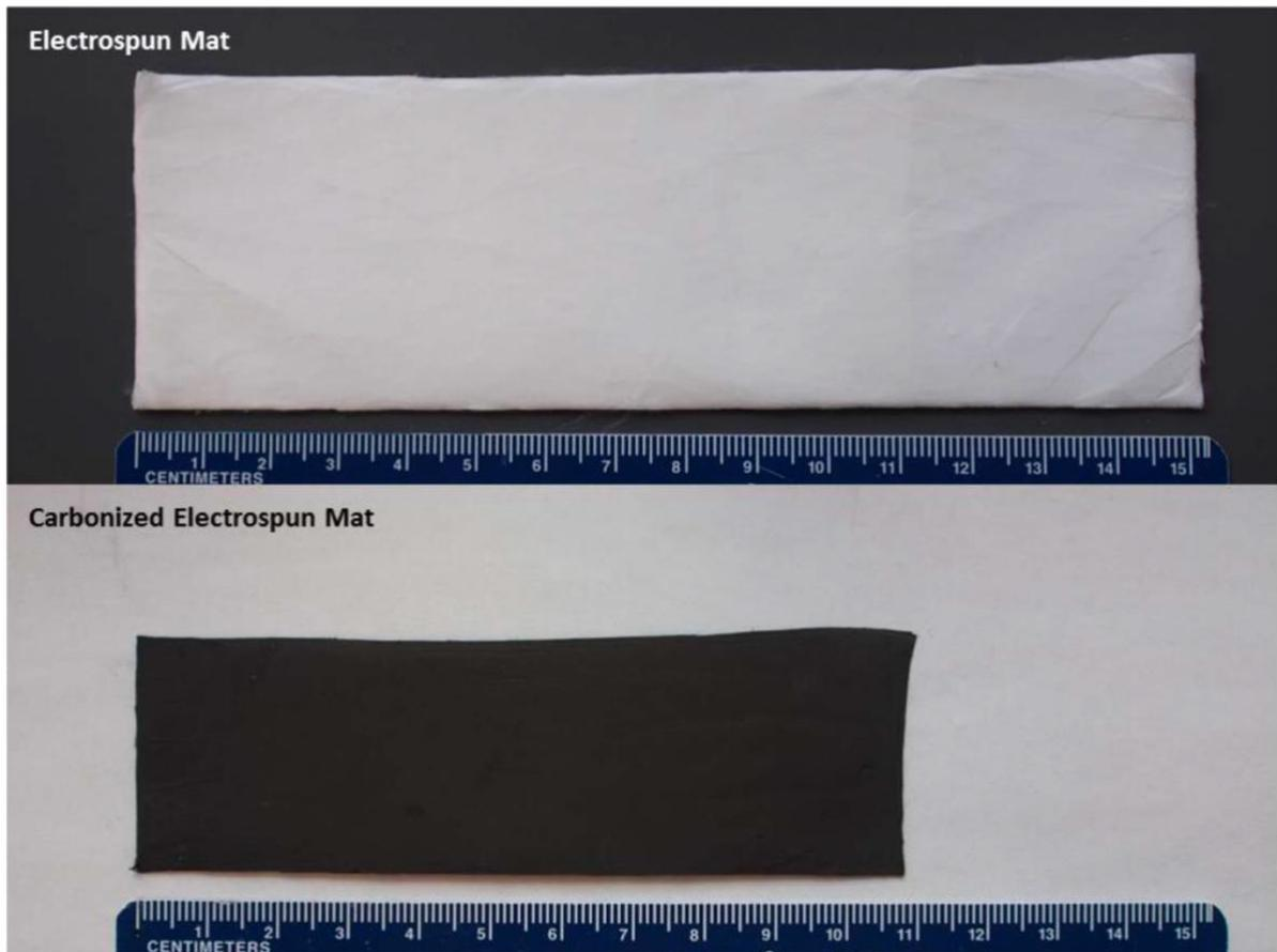
**Figure 2-7 - Electrospun polyacrylonitrile (PAN) material before and after carbonization [24]**
