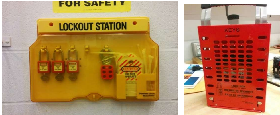
Figure 7: Lockout Station and Corresponding Lockout/Tagout lockbox
