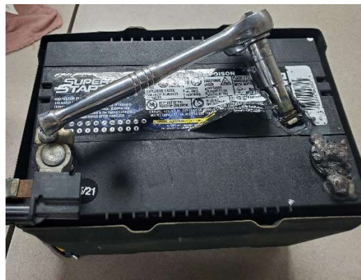
Figure 24: Unprotected battery leads destroyed by dropped wrench [35]
