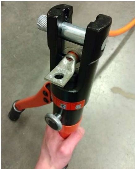
Figure 13: HV wire in a crimping tool
