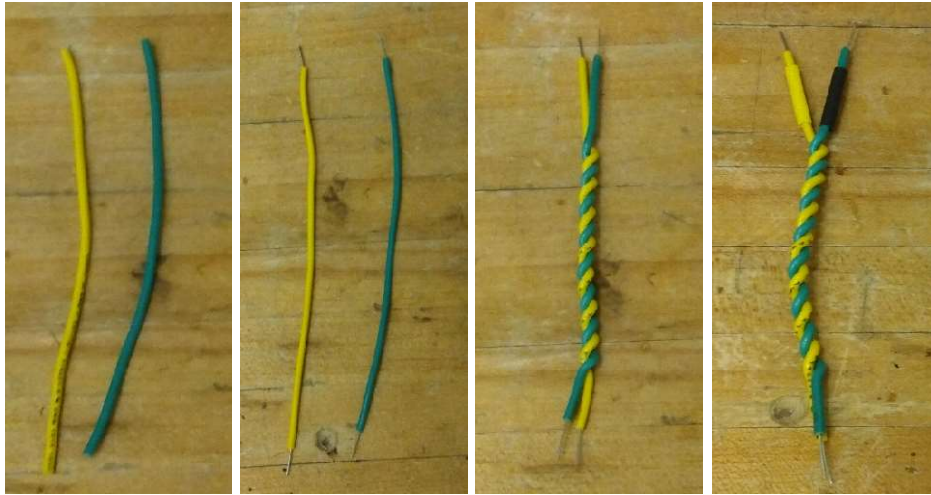
Figure 49: CAN Wire Building Steps 1-3
