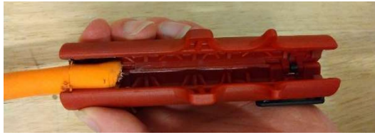
Figure 11: Stripping insulation and shielding from an HV cable
