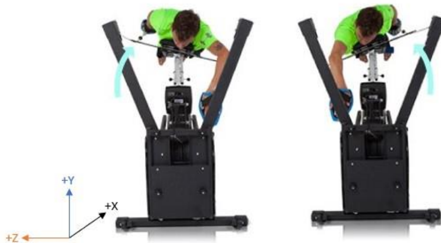
Figure 11. Kayak Pro SwimFast swim bench rotation allowance on rotating bench (SwimFast Ergometer, n.d.). Kayak Pro SwimFast swim bench used for collections was an older model than pictured and did not include the Halo™ Swim Trainer Template or the full palm handles.
