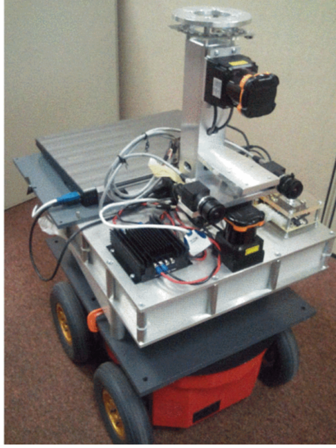
Figure 2.1: Mobile wheeled robot with LiDARs and computing unit [38]
