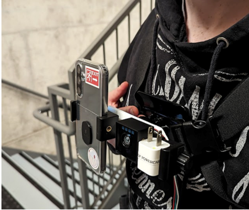
Figure 4.7: Cygbot Cyglidar D1 collection mount design with accompanying phone for validation
