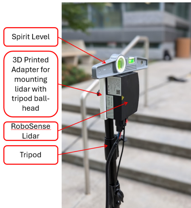
Figure 4.9: Tripod setup for the RoboSense RS-LiDAR-M1 v2 sensor, featuring a 3D printed adapter for secure mounting, a spirit level for precise alignment, and a stable tripod for stationary data acquisition.
