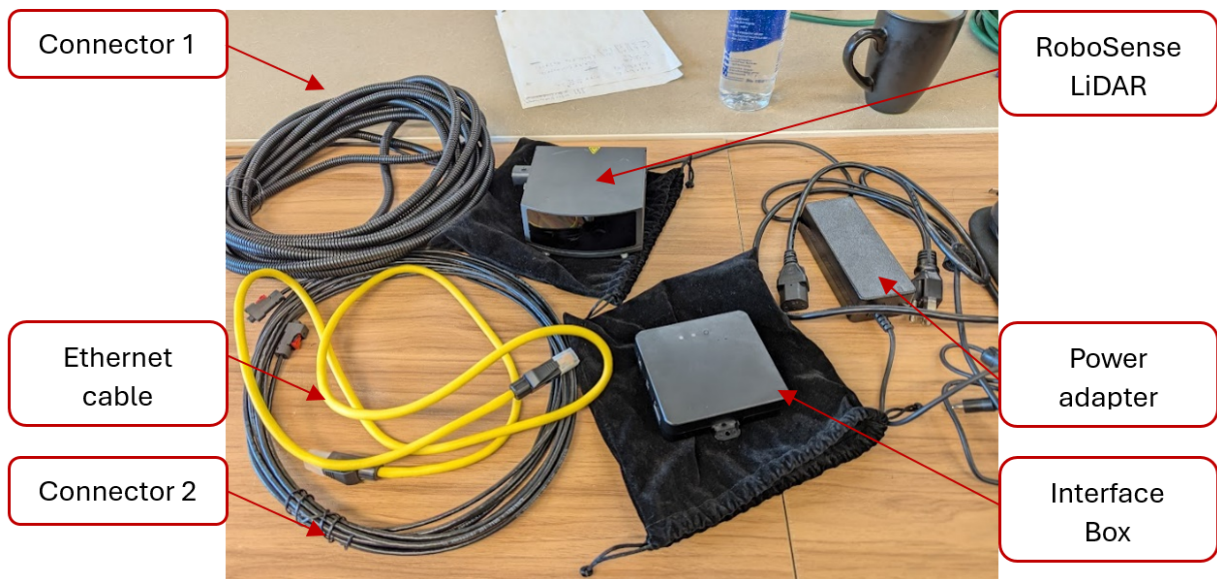
Figure 4.4: Essential components Involved connecting the RoboSense LiDAR [51].
