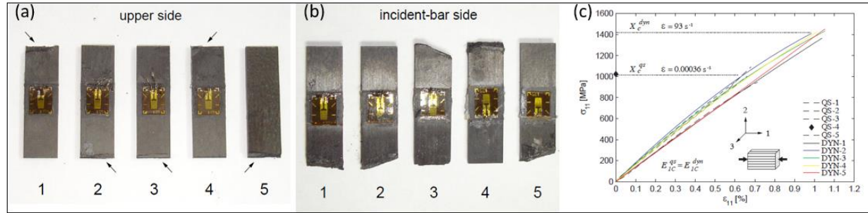
Figure 2-6: Images of the failed specimens tested at: (a) quasi-static strain rate [17], and (b) high strain rate [17]. (c) Stress-strain response for specimens tested in longitudinal compression at quasi-static and high rates [17].
